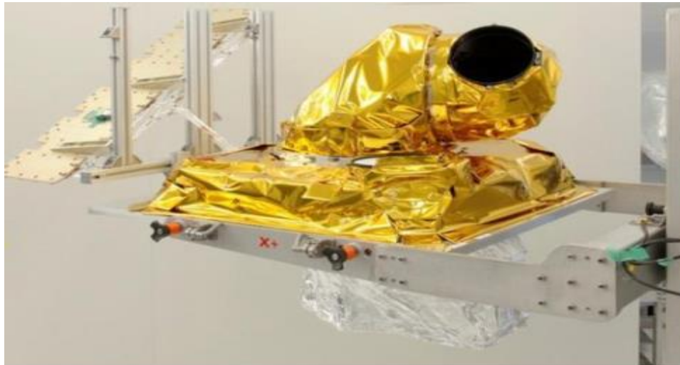
Figure 9: Alphasat LCT before integration into the Spacecraft.
