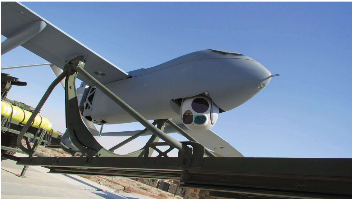
Figure 35 – View of the Aerosonde EO sensor while the drone is on the launch catapult (Textron Systems 2021). This component will be replaced by the acquiring and tracking device. All the other components will be accommodated inside the drone.
