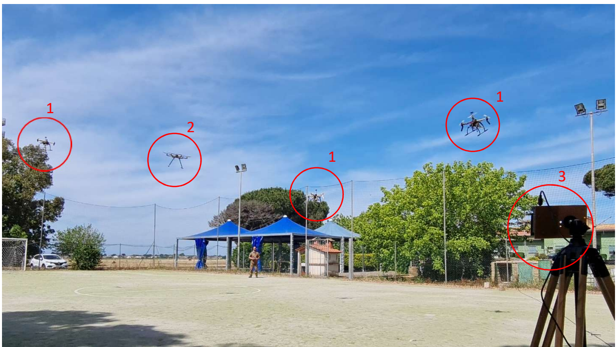
Figure 6 – Swarm activity at Italian Flight Test Wing – A swarm of three mini-class decoy drones (1) mask an allied drone (2) from a 24GHz radar (3) (Verini Supplizi, et al. 2021)
