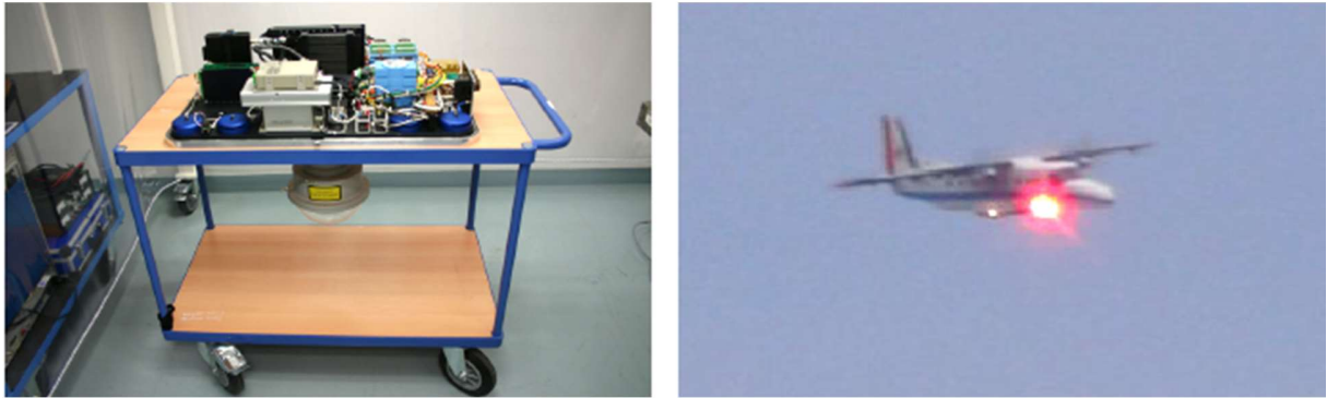
Figure 18 - Left: Optical Terminal in Lab. Right: View of Do228 aircraft firing its laser during trials (Fuchs e Giggenbach 2010)
