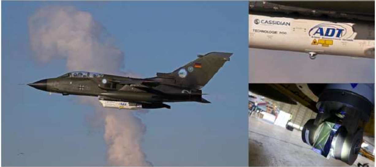
Figure 30 - Left: Tornado with attached ADT-Pod during the second flight test. The white long box is the ADT-Pod with integrated MLT. (Source: Josef Gietl/Airbus Defense & Space). Upper right: close-up of the ADT-Pod revealing the MLT dome. Lower right: MLT CPA without glass dome during inspection (Source: ViaLight Communications). (Moll 2014)
